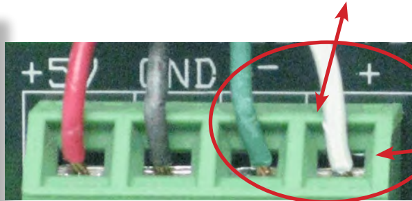
Enlarged view of Thermostat block wiring
