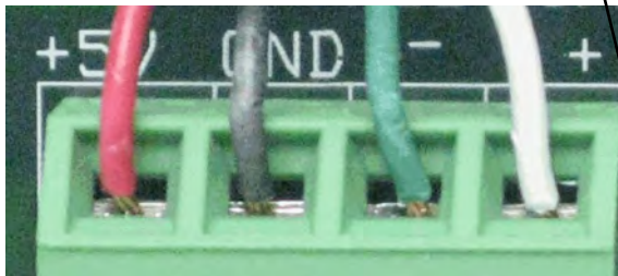
Enlarged view of Thermostat block wiring
